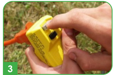
3 Press "TEST" Button To Verify GFI Function, Then Press "RESET"
